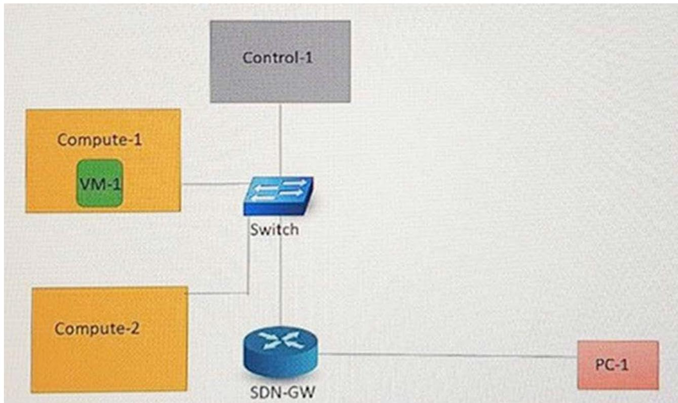
Virtual machine VM-1 is spawned on a compute node Compute-1. VM-1 is not able to ping PC-1, which is located outside of the SDN cloud. You want to run packet captures to trace the packet initiated by VM-1 towards PC-1.
